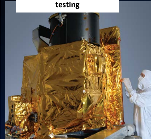
ABI FM1 completed vib testing
