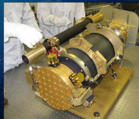
SUVI FM1 beginning environmental testing
