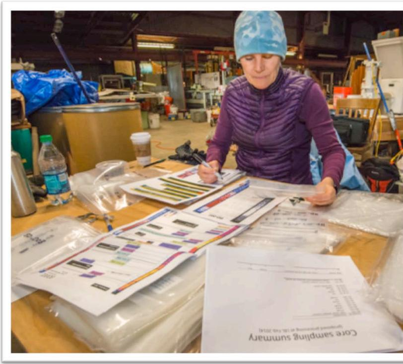
*Cathy Wilson (LANL) annotating the CT scan image and labeling sample bags. CT images were annotated with sample analysis information and sample depth intervals in preparation for sub-sampling with the chop saw in the cold lab. Photo credit Roy Kaltschmidt (LBNL).*
