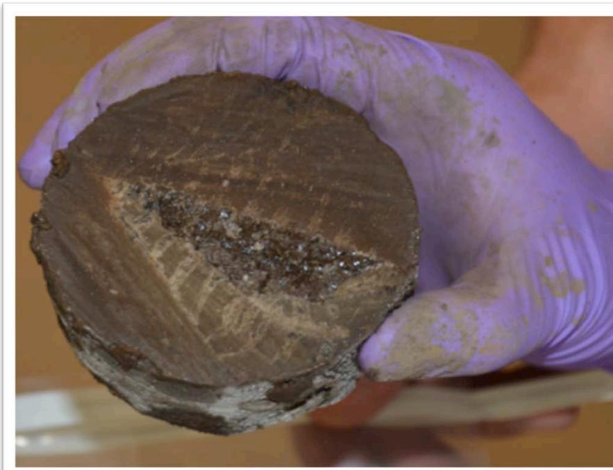
*Sectioned NGEE Arctic core sample from the center of a transitional polygon showing a brown mineral silty sand appearance with porous cryostructure and an ice inclusion. Photo credit Roy Kaltschmidt (LBNL).*
