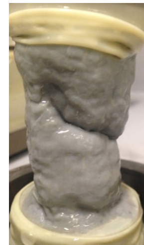
End of analyses; noticeable shrinkage and creases in sample
