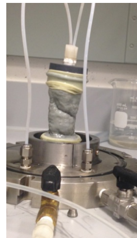
End of analyses; noticeable shrinkage and creases in sample
