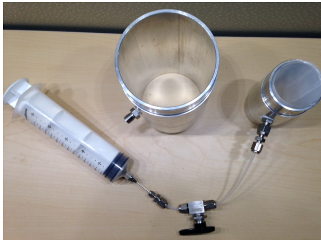
Figure 5. Top-view of cylindrical membrane stretchers with 3.5''-inside diameter (left) and 2.0''-inside diameter (right) attached to a 140-cc syringe
