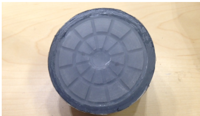
Figure 3. End cap with nylon mesh netting glued to the top.
