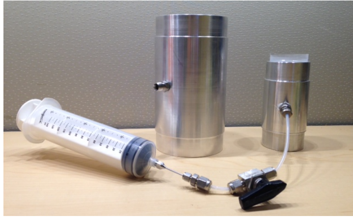
Figure 4. Side-view of cylindrical membrane stretchers with 3.5''-inside diameter (left) and 2.0''-inside diameter (right) attached to a 140-cc syringe
