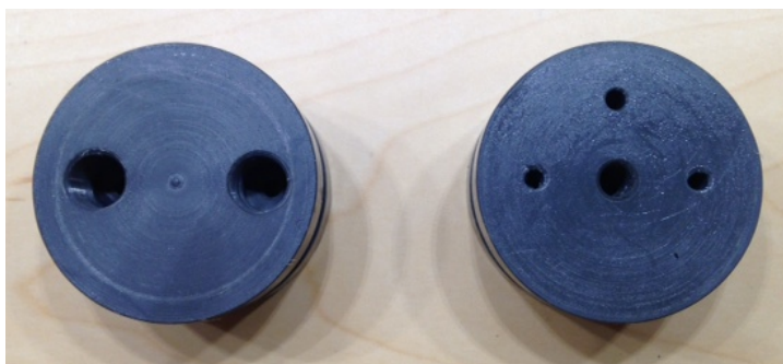
Figure 2. Reverse sides of each end cap with holes for fittings to connect to the “upper” valves of the permeameter (left) and holes for “lower” valve flows, a center screw-hole to secure the bottom end cap to the bottom plate and a small hole for the reference pin (right).
